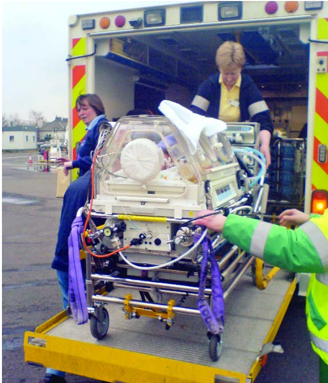
FIGURE 4 Loading the incubator into the ambulance using the tail lift.
