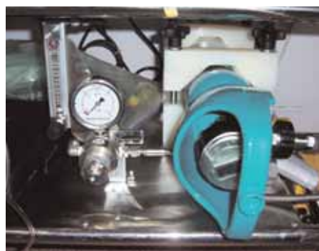
FIGURE 3 Close up of the iNO cylinder, regulator and flowmeter.
