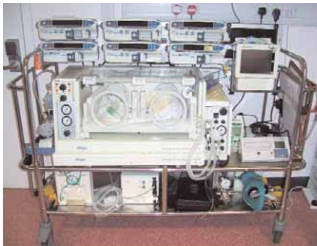
FIGURE 2 The ANTS transport incubator with iNO delivery and monitoring equipment mounted.
