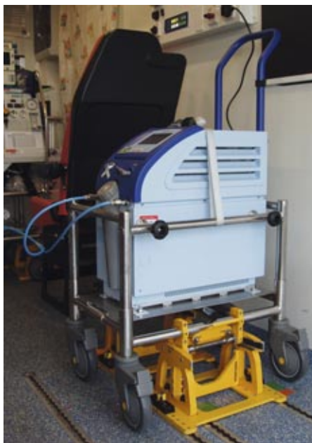
FIGURE 2 Servo-controlled cooling unit mounted in a wheeled cage and secured within the ambulance.
