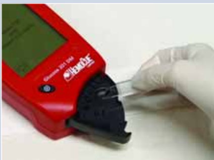
FIGURE 7 The microcuvette is then placed in the holder and inserted into the photometer.
